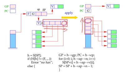
The instruction apply unpacks the F-object, a reference to which (hopefully) resides on top of the stack, and continues execution at the address given there:
